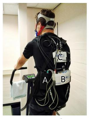
**Figure 3.2** Attachment of the VU-AMS and Cosmed K4b<sup>2</sup>. A) VU-AMS; B) Cosmed main unit; C) Battery pack.
